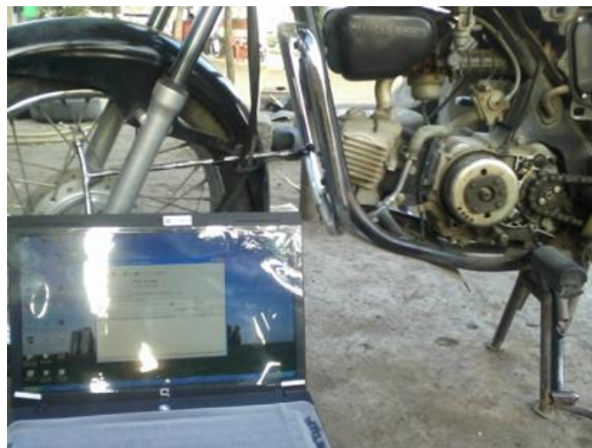
Fig. 3: Experimental Setup with audio signal capturing system
