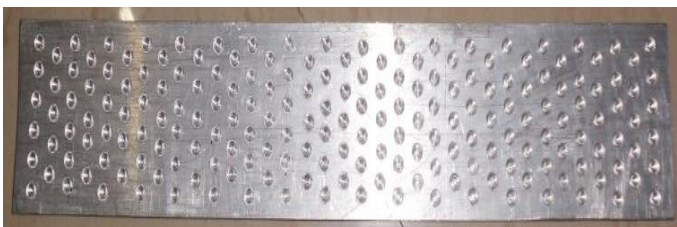
Fig.8: original dimpled plate with staggered arrangement
