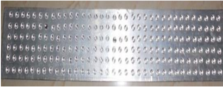
Fig.6: original dimpled plate with simple arrangement
