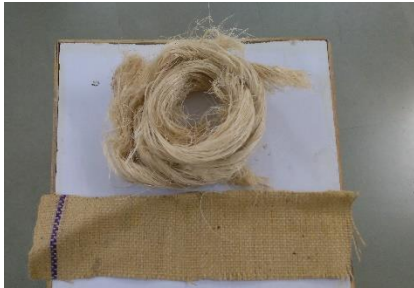
Fig.1.Raw natural fiber (Banana & Jute).
