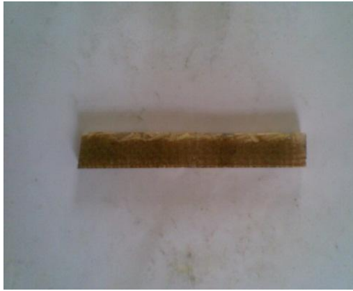
Fig.10.Flat bar shape for flexural testing.
