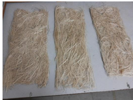
Fig.4. Multi direction pattern of banana fibre.
