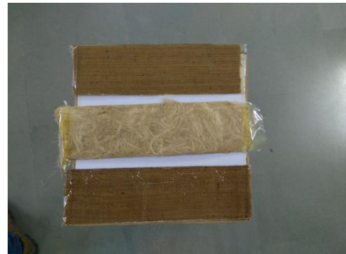
Fig.8.Bnana & Jute composite fibre sample.
