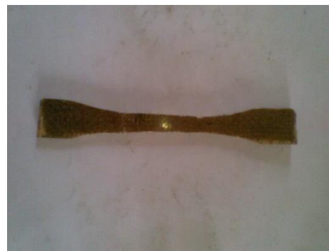
Fig.9.Dog bone shape for tensile testing.
