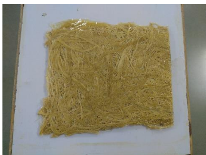
Fig.6.Banana composite fibre sample.
