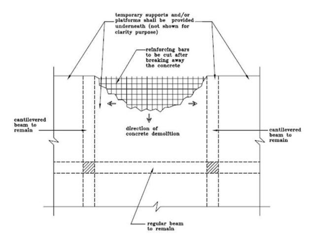
away the concrete. The reinforcement shall remain and be cut off after the concrete is broken away
