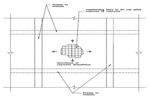
area within reach of the rope or tie wire. The concrete shall be broken away first before the cutting of reinforcement. Alternatively the reinforced concrete slab may be cut by saw cutting. Demolition sequence would be as shown in following figures.
