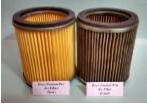
Fig. 1.1: Comparison between new air filter and clogged filter
