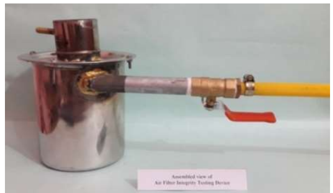
Fig. 5.4: Air Filter Integrity Testing Device
