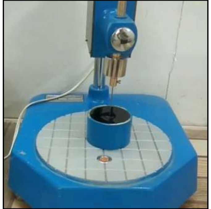
Fig. Penetration Test
