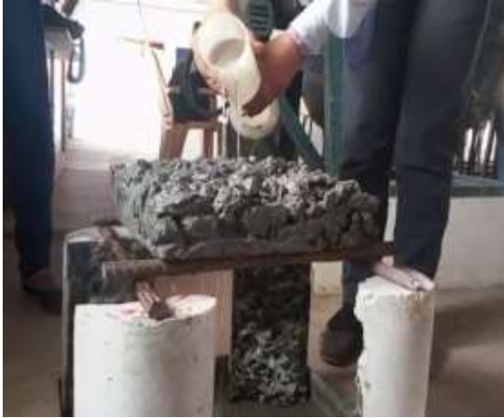
Fig. No 4 Sample for the infiltration test
