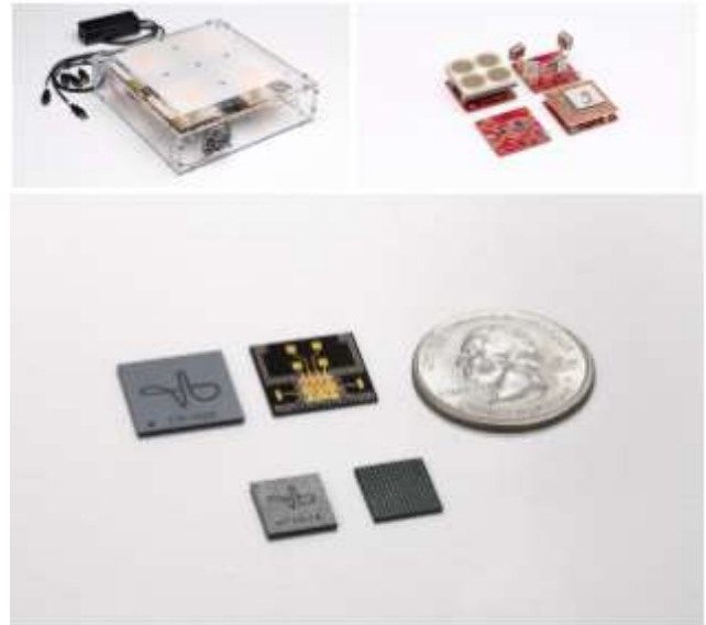
Fig-4: Top: Early prototypes of Soli FMCW and impulse radars. Bottom: Soli radar 60 GHz chips with antennas-in-package (AiP).
