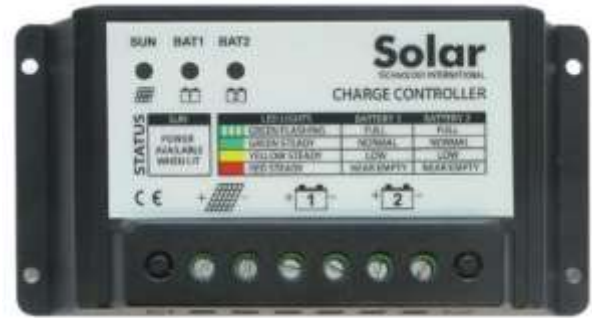
Fig-3: Charge Controller
