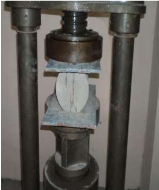
Fig 3 : Split tensile test on cylinder
