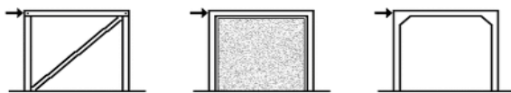
Three basic methods of assuring lateral stability of simple structural assemblies: diagonal bracing, shear planes, and rigid joints
