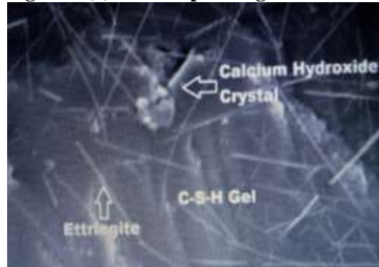
Figure.4.(b)microscopic image of concrete with copper slag and magnetized water
