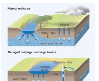
Natural recharge is precipitation, river bed seepage, flooding and other natural forms of water that enter the groundwater system. Artificial aquifer recharge is the enhancement of natural groundwater supplies using man-made conveyances such as infiltration basins, field flooding, infiltration galleries or injection wells. Often, AR is conducted to improve groundwater resources (i.e. increasing storage) and is often incorporated into a broader water resource plan.
