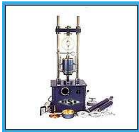
Fig 5 Testing of CBR specimen
