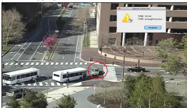
Fig.2.1.1 Vehicle in wrong direction
