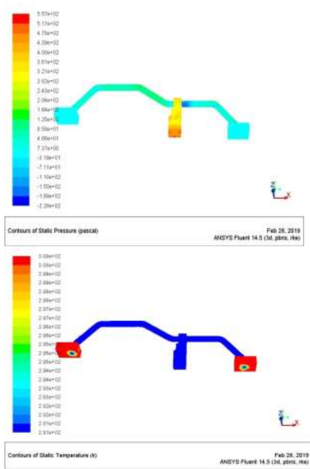
Figure 3.4: Pressure and Temperature counter obtained through CFD Analysis.
