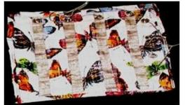
Fig-3.2(a): Fabric switching contact keyboard
