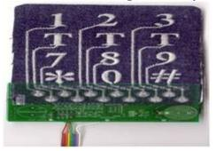
Fig-3.2(b): Capacitive keyboard
