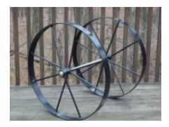
**2)** Shaft/axel:- It is long circular part of metal which mainly use to connect driving wheels . also it contain gear\ pinion to transfer the driving motion from driving wheel to another pinion .
