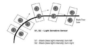
Fig 3: Module of Line Sensing
