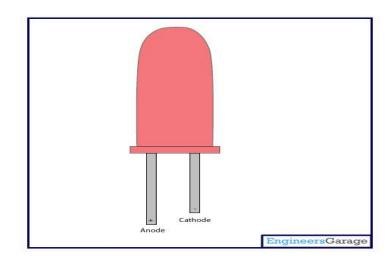
Fig 7: Pin Diagram LED
