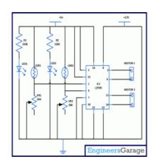
Fig 9: Circuit diagram by using L293d
