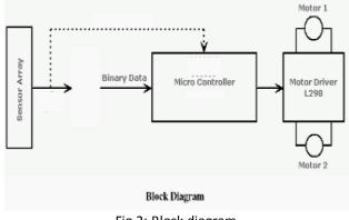
Fig.2: Block diagram
