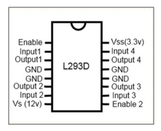
Fig 6:-Pin Diagram L293d
